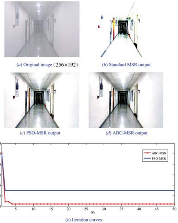
**Fig. 6.** Comparison results of the MSR algorithms in Scene 4. (a) Original image (256 × 192). (b) Standard MSR output. (c) PSO-MSR output. (d) ABC-MSR output. (e) Iteration curves.
