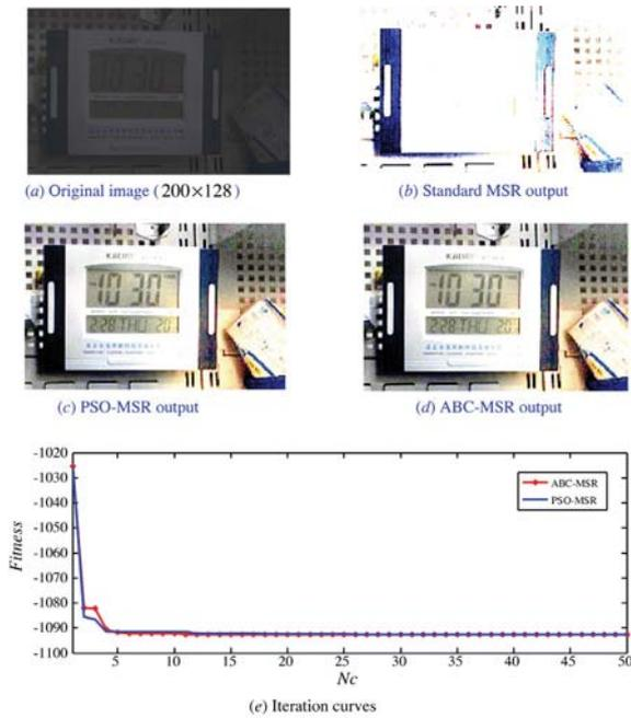
**Fig. 4.** Comparison results of the MSR algorithms in Scene 2. (a) Original image (200 × 128). (b) Standard MSR output. (c) PSO-MSR output. (d) ABC-MSR output. (e) Iteration curves.
