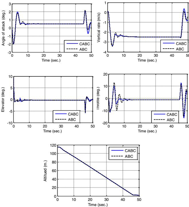
Fig. 7. Results of tuned controller parameters for automatic landing system based on ABC and CABC.
