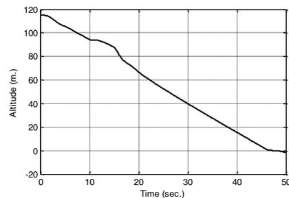
Fig. 10. Aircraft altitude response with turbulence.
