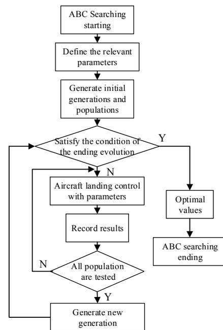
Fig. 6. The automatic landing system parameters tuning process based on CABC.
