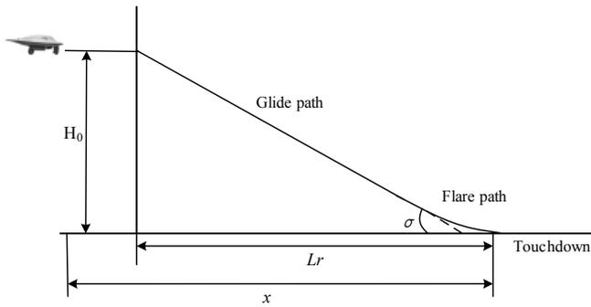
Fig. 1. The reference landing trajectory.
