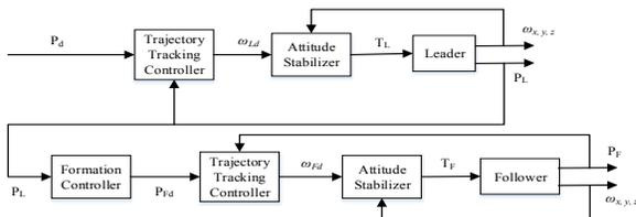
Figure 1. Trajectory tracking control strategy block diagram.
