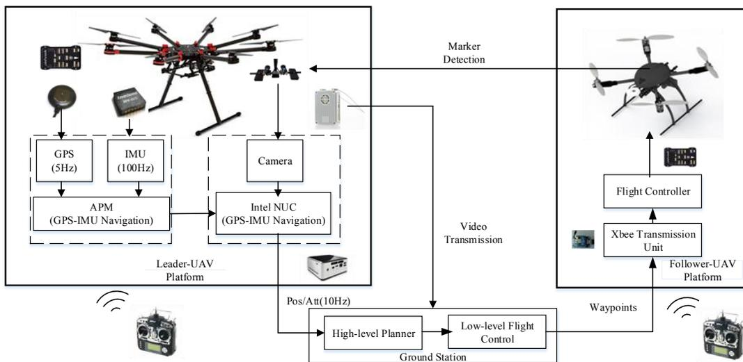
Figure 3. Hardware architecture of our UAV platforms.
