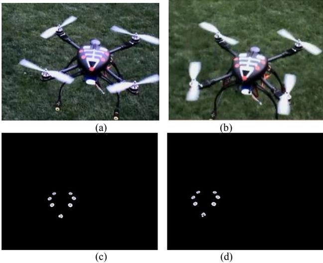
Figure 5. Results of marker detection. (a)–(b) Cooperative markers on the follower-UAV. (c)–(d) Segmentation results of left camera and right camera, respectively.
