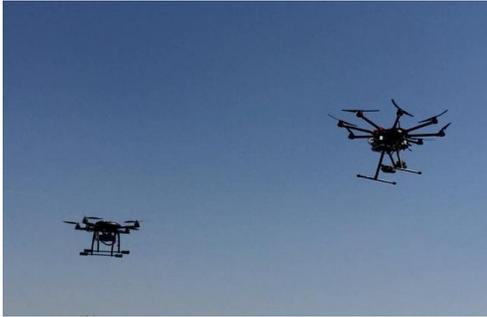
Figure 4. Outdoor formation control experiment based on visual measurement and IMU data.
