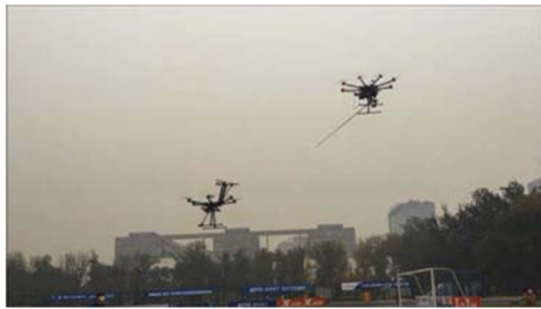
Fig. 4. Leader-follower formation flight platform used in Experiment II.
