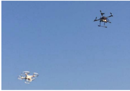
Fig. 7. Leader-follower formation flight platform used in Experiment III.
