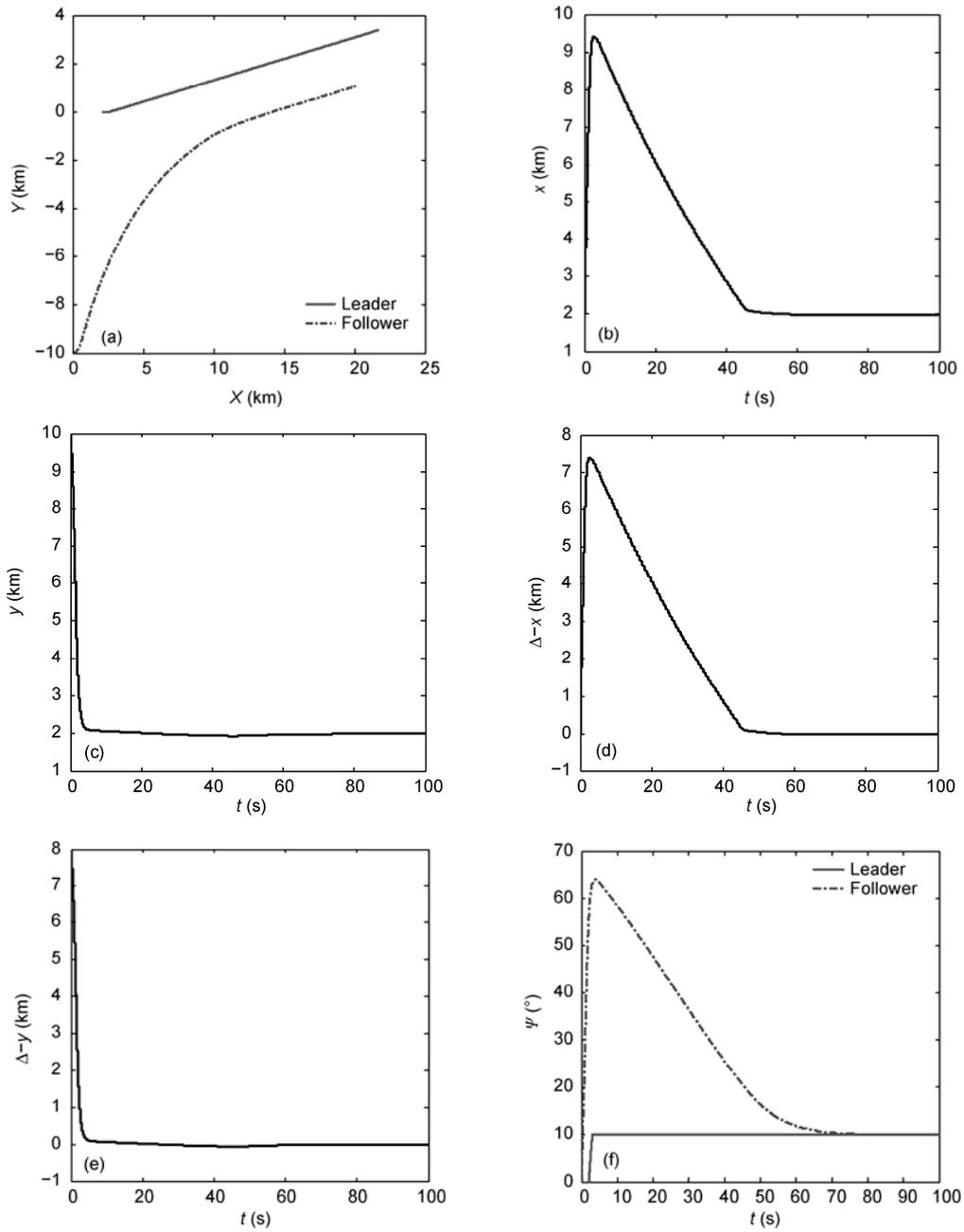
**Figure 7** Experimental results of formation based on PD controller. (a) Flight trajectories of leader-follower formation; (b) Relative distance ( $x$ ) of X-axis; (c) Relative distance ( $y$ ) of Y-axis; (d) Deviation distance ( $\Delta x$ ) of X-axis; (e) Deviation distance ( $\Delta y$ ) of Y-axis; (f) Responses of heading angle ( $\Psi$ ).
