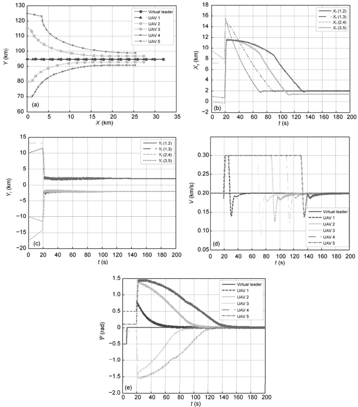
**Figure 8** Experimental results of formation flight. (a) Five UAVs merge to a V-formation while following a virtual leader; (b) Relative distances ( $X_r$ ) of X-axis; (c) Relative distances ( $Y_r$ ) of Y-axis; (d) Velocity ( $V$ ) responses of five UAVs; (e) Heading angle ( $\psi$ ) responses of five UAVs.
