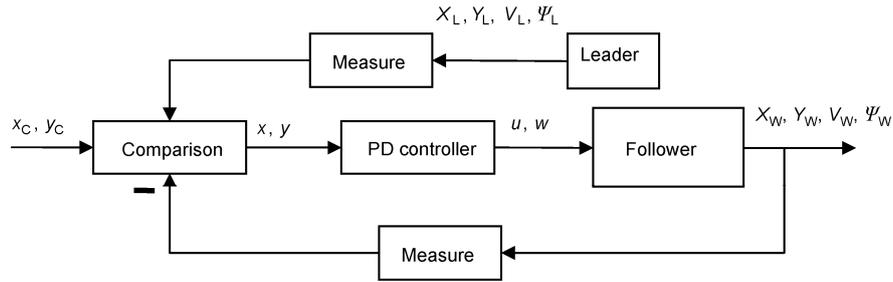
**Figure 3** System structure for UAV leader-follower formation control, where  $x_c, y_c$  are expectations of relative distance,  $x$  and  $y$  denote the actual distance,  $u$  and  $w$  are control inputs generated by PD controller.
