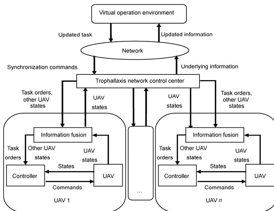
Figure 1 Multiple UAVs formation flight system based on trophallaxis network control.
