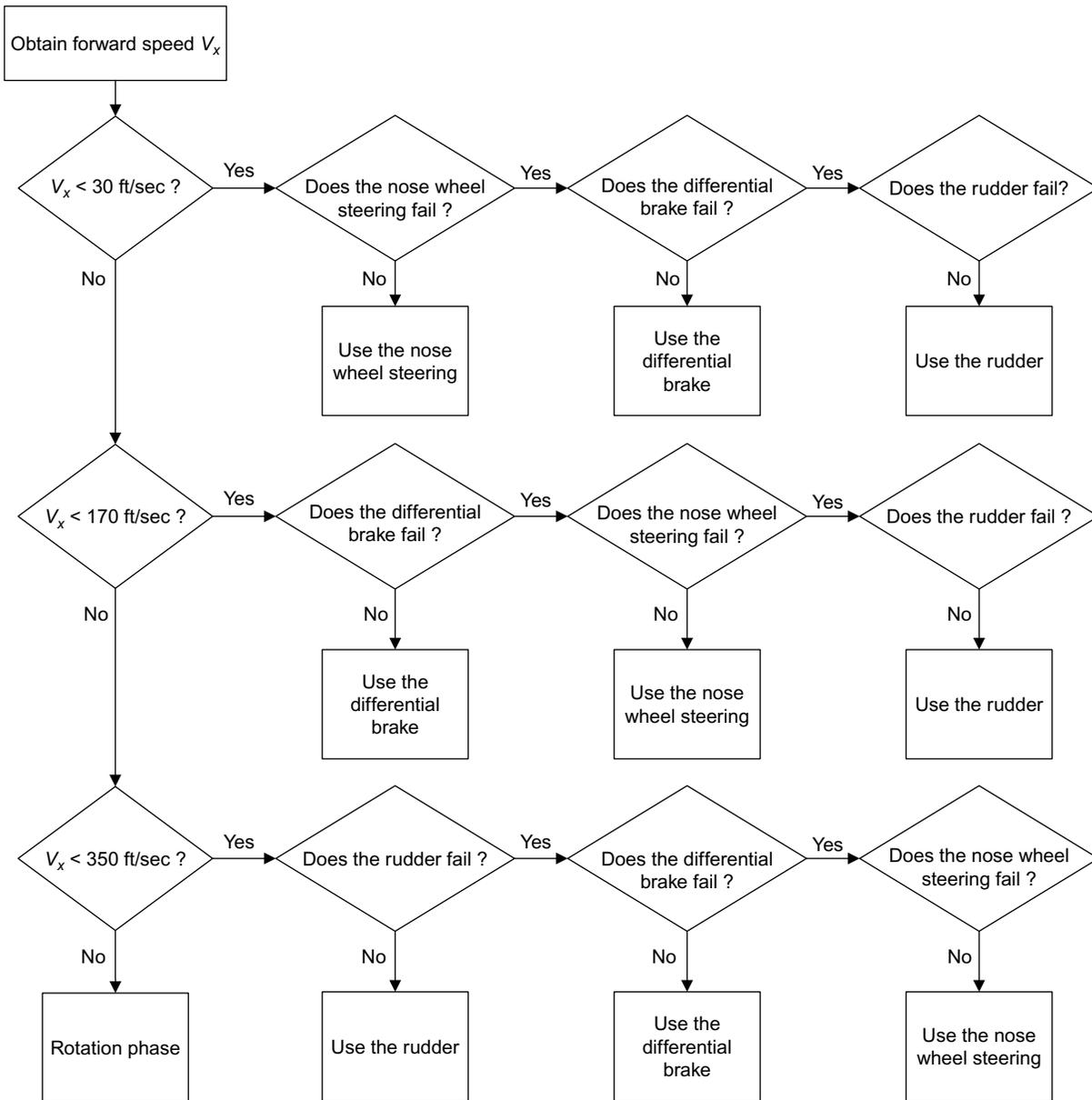
In the simulations, the low speeds range from 0 to 30 ft/s, the medium speeds from 30 to 170 ft/s, and the high speeds from 170 to 350 ft/s. The rotation speed is 350 ft/s. The crosswind is a 50 ft/s constant wind which is perpendicular to the runway centreline, and this satisfies the relevant criteria stated in MIL-HDBK-1797.
