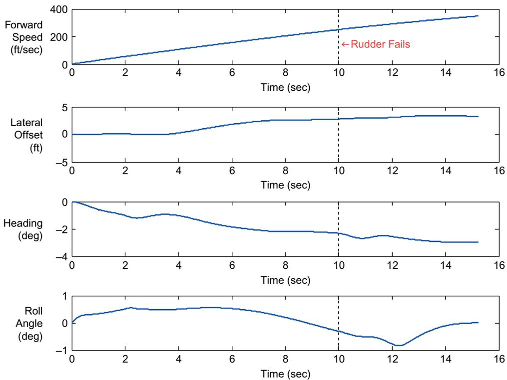
Figure 11 Input variables in rudder failure condition simulation
