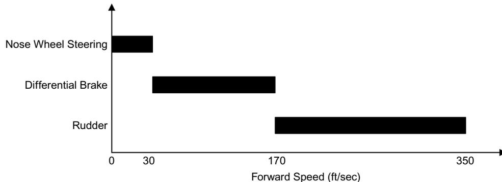
Figure 4 Switch between different control devices during takeoff roll
