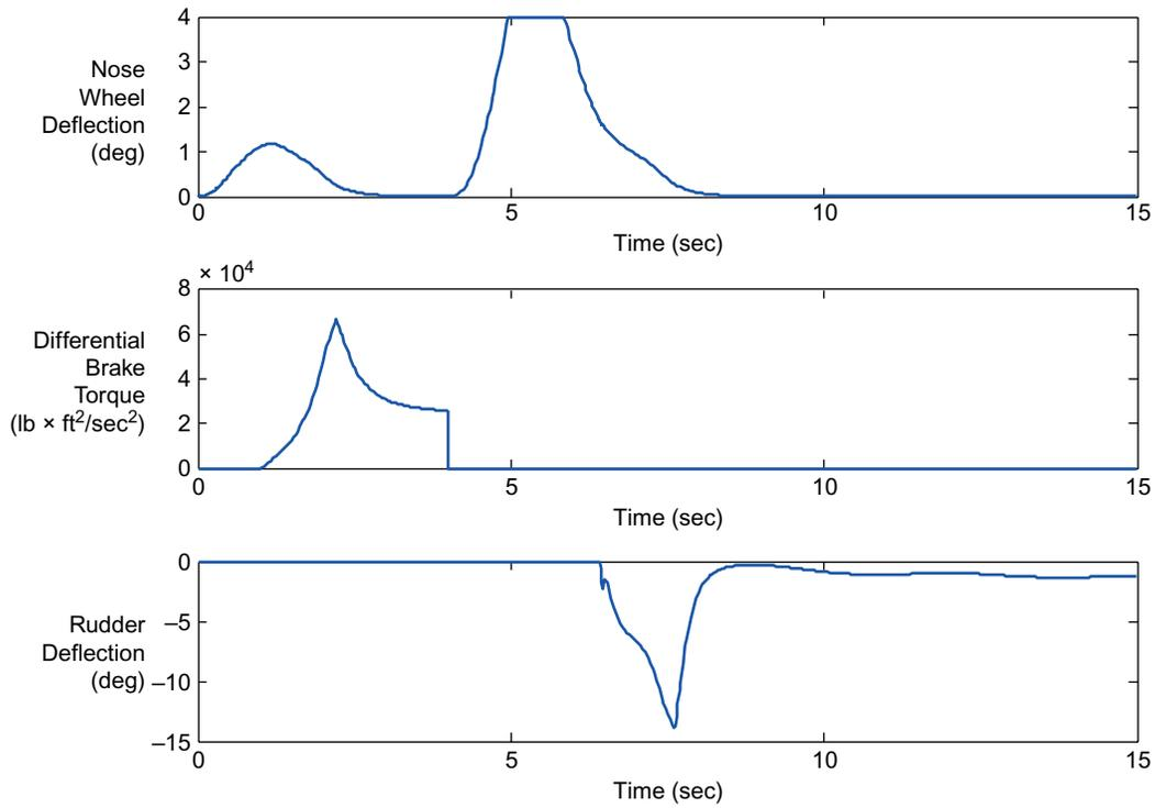
Figure 10 Response of state variables in rudder failure condition simulation
