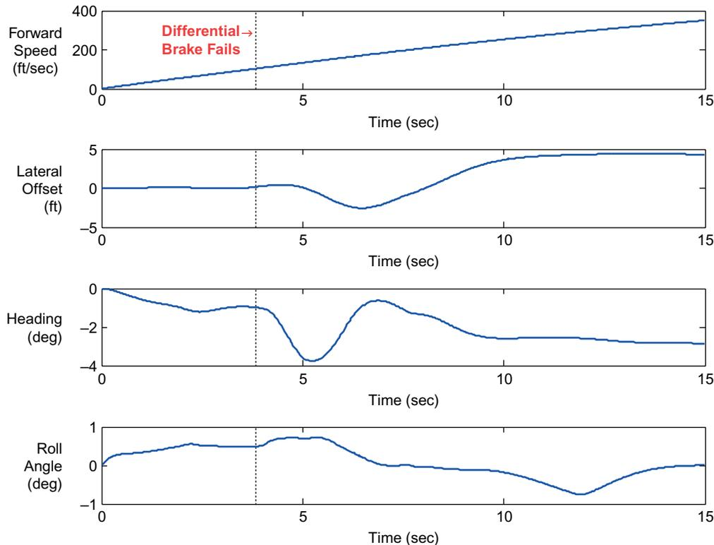
Figure 9 Input variables in differential brake failure condition simulation
