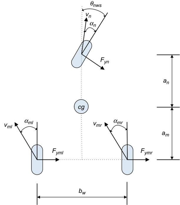
where  $a_n$  is the distance between the nose tire to UCAV centre of gravity along body x-axis.
